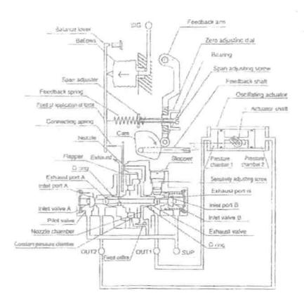
Counter operation is available by setting the cam back to front and connect pepings of OUT1 and OUT2 contransise.
